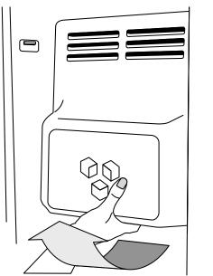
If the icebox cannot be easily fitted, remove it and turn the corkscrew mechanism 90°. Then reinstall the icebox, ensuring that the catch pin on the tray fits into the slot on the shelf.
